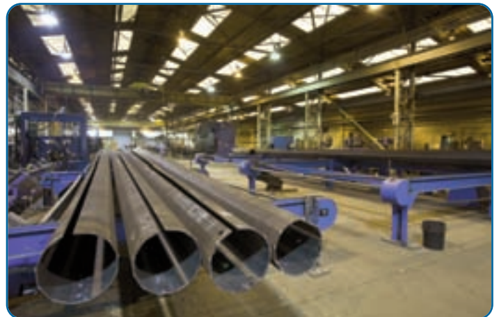
Formed tube sections fresh from being processed on the new press wait to be fed into the new long seamer. The formed sections move from the press to the long seamer on a transfer table designed and built by T&B employees.
