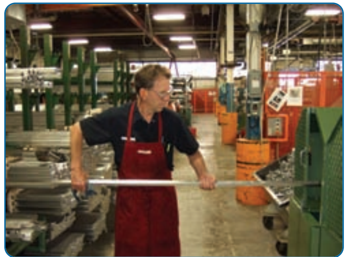
Yves Leblanc, machinery operator, demonstrates how the 12 foot aluminum bar is inserted into the machine.
