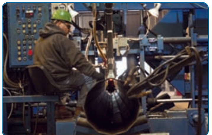
Jeff Sigmon monitors the new seam welder to ensure top quality welds.
